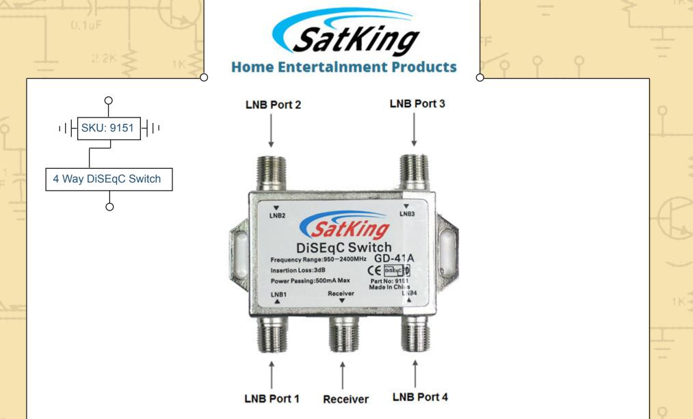
This DiSEqC switch is to connect up to four dishes into one receiver. Simply go into LNB setup in your receiver and for the first satellite select port 1 and for the second satellite select port 2 and the same for port 3 and 4. No power injector is required for this DiSEqC switch as the power is provided by the satellite receiver.
