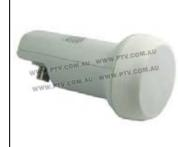
11300 Ku Offset Dual Polarity RF:12.25-12.75 GHz L.O. 11.3 GHz IF:950-2050 MHz Noise 0.5 dB
